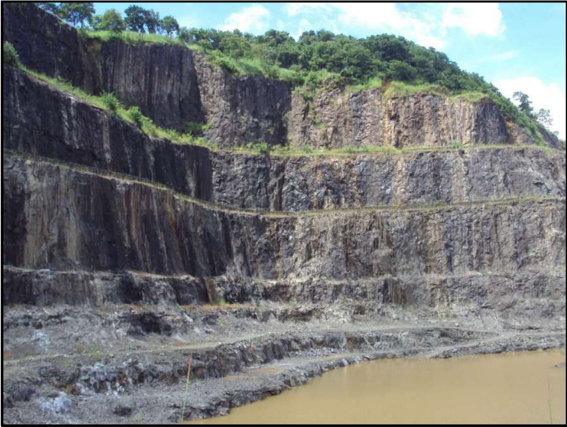
Photograph showing the bench type mining
